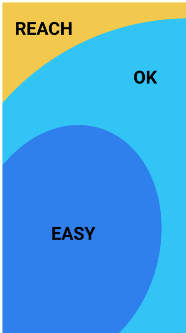
PICTURE 5. Touch area of phone. For a right-handed user. (Wroblewski 2011 - Redrawn Keogh 2020)
