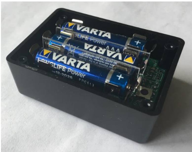
Figure 22: The prototype with batteries inside the cover box
