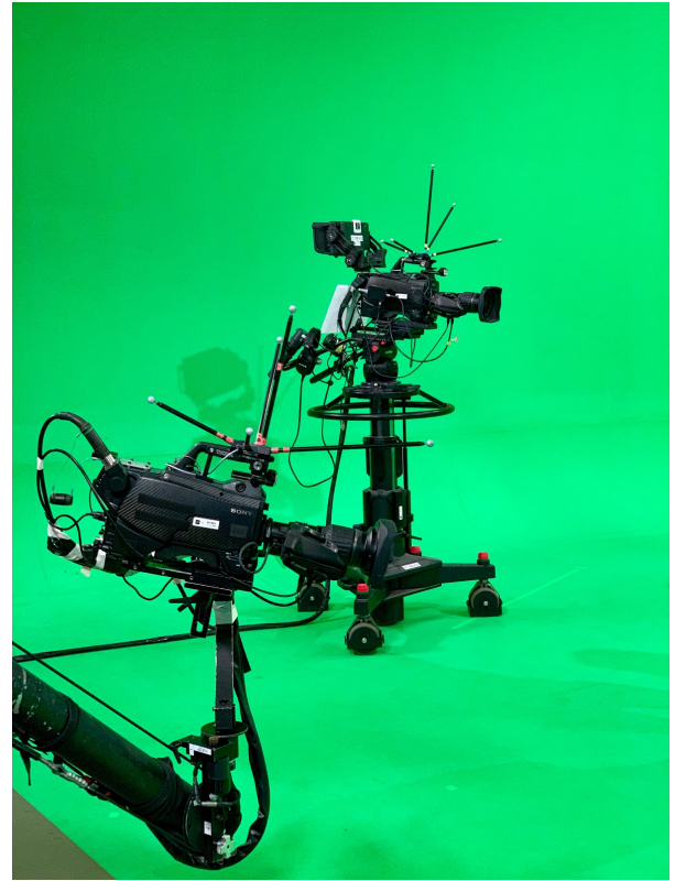
PICTURE 7. Studio cameras tracked with a motion capture system.
