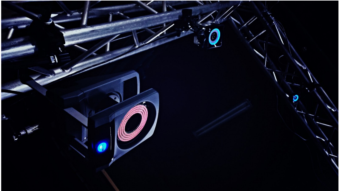
PICTURE 6. Motion capture cameras attached to the truss system at the motion capture stage.
