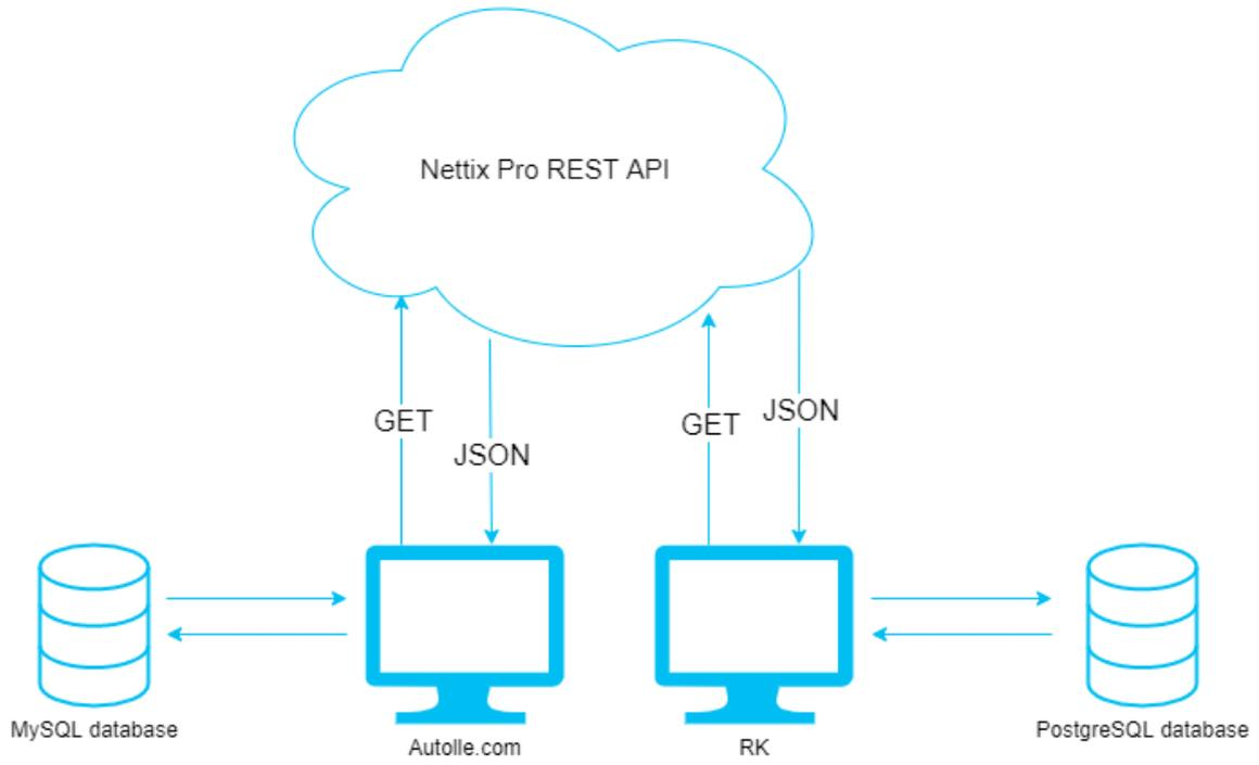
FIGURE 5. How Autolle.com and RK websites use Nettix Pro REST API
