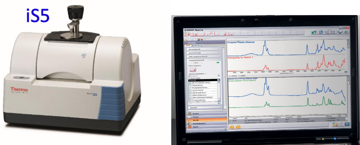
Figure 11: FTIR analysis equipment used for experiment in Arcada laboratory
