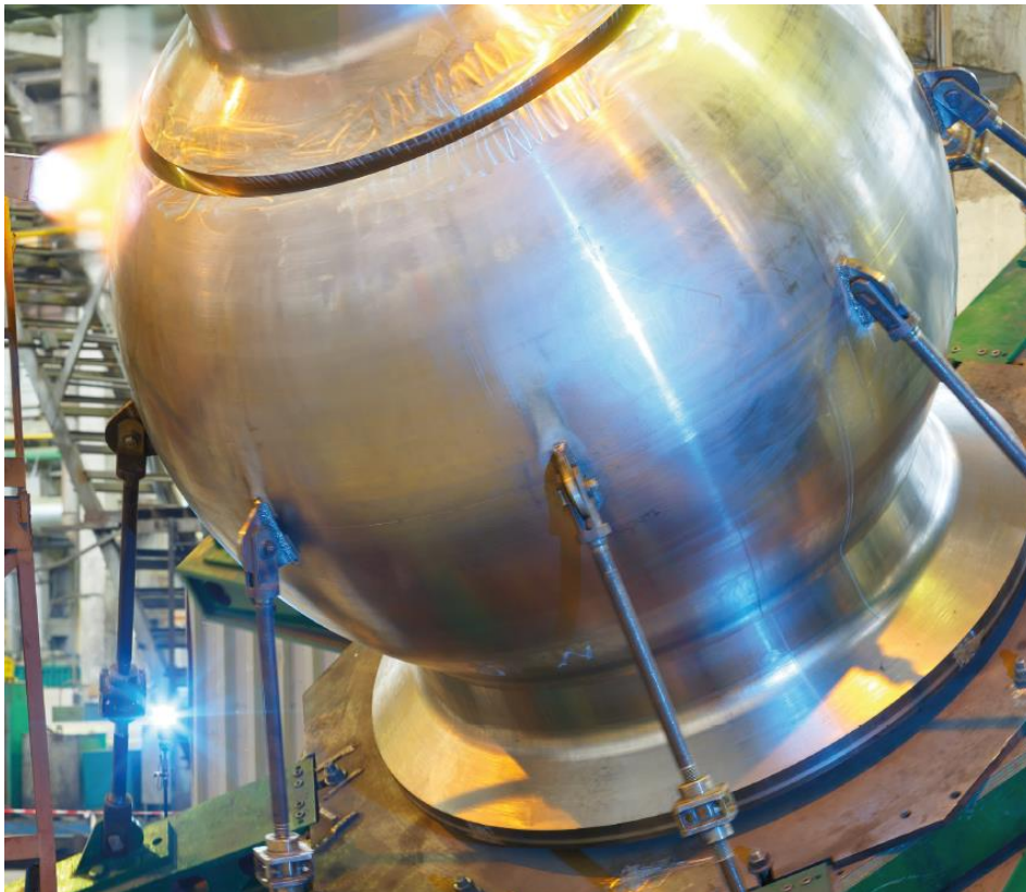
FIGURE 9. Temporary attachments welded to main coolant pump spherical housing for fixing to positioner (AEM-technology JSC. Equipment for nuclear power industry. p. 12)
