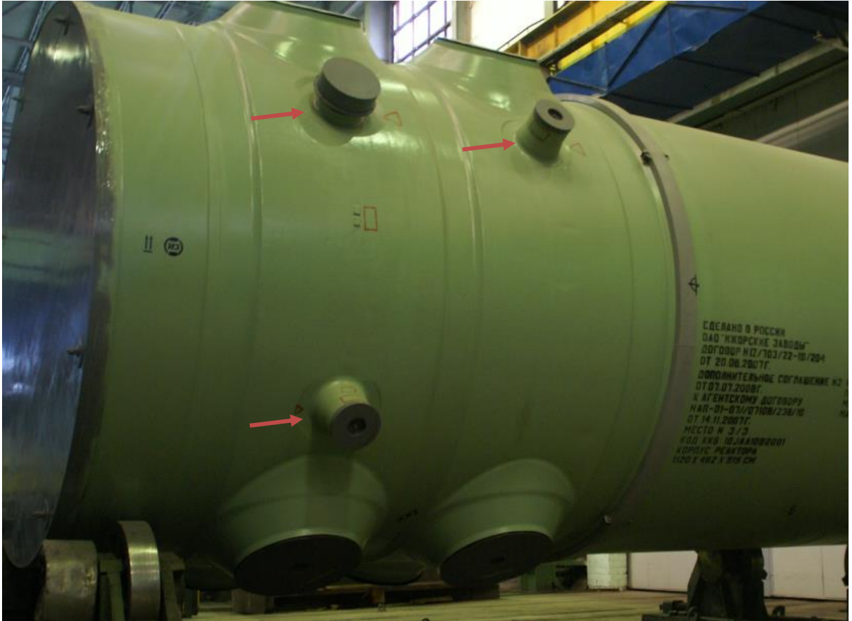
FIGURE 7. RPV set-on nozzles (pointed out with arrows) (adapted from VVER-1200 RPV retrieved 2.6.2020 http://www.omz.ru/en/company/project/project1/ )
