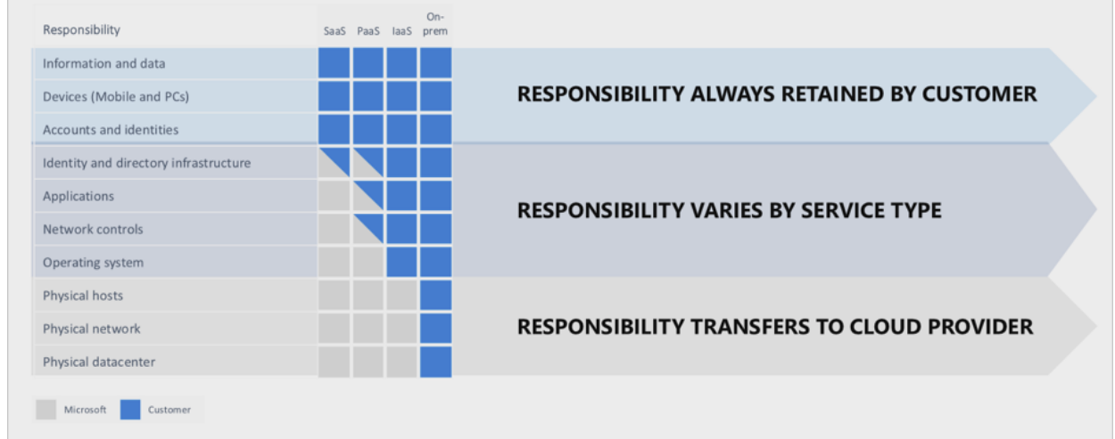
Figure 12. Security responsibilities between the service models. (Microsoft Shared responsibility in the cloud 2019.)
