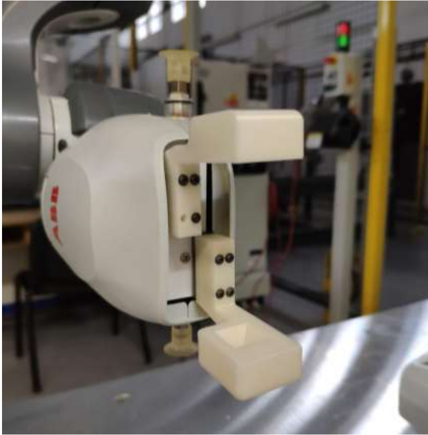
Figure 7 shows The designed finger gripper was inserted on the right gripper
