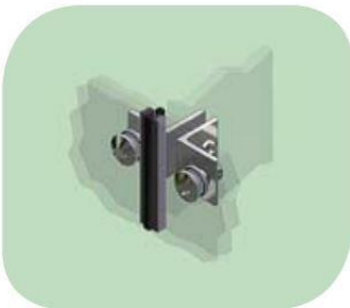
Pilkington Planar ™ Intrafix insulated double glazed unit with standard angle spring plates.
