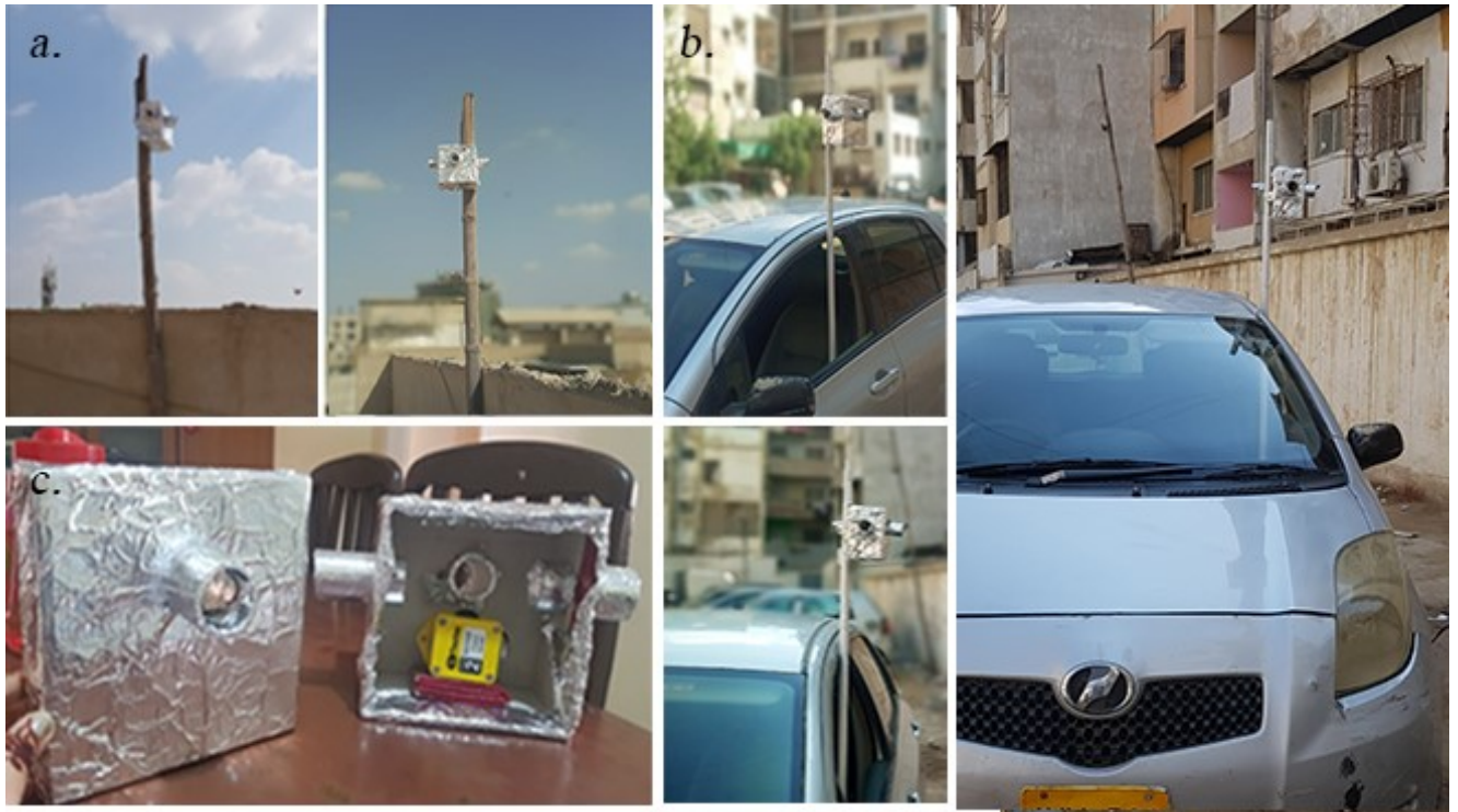
Figure 9. (a) Device mounted on the fixed location, (b) mobile stations and (c) the insulated and ventilated cardboard box for daytime surveys.
