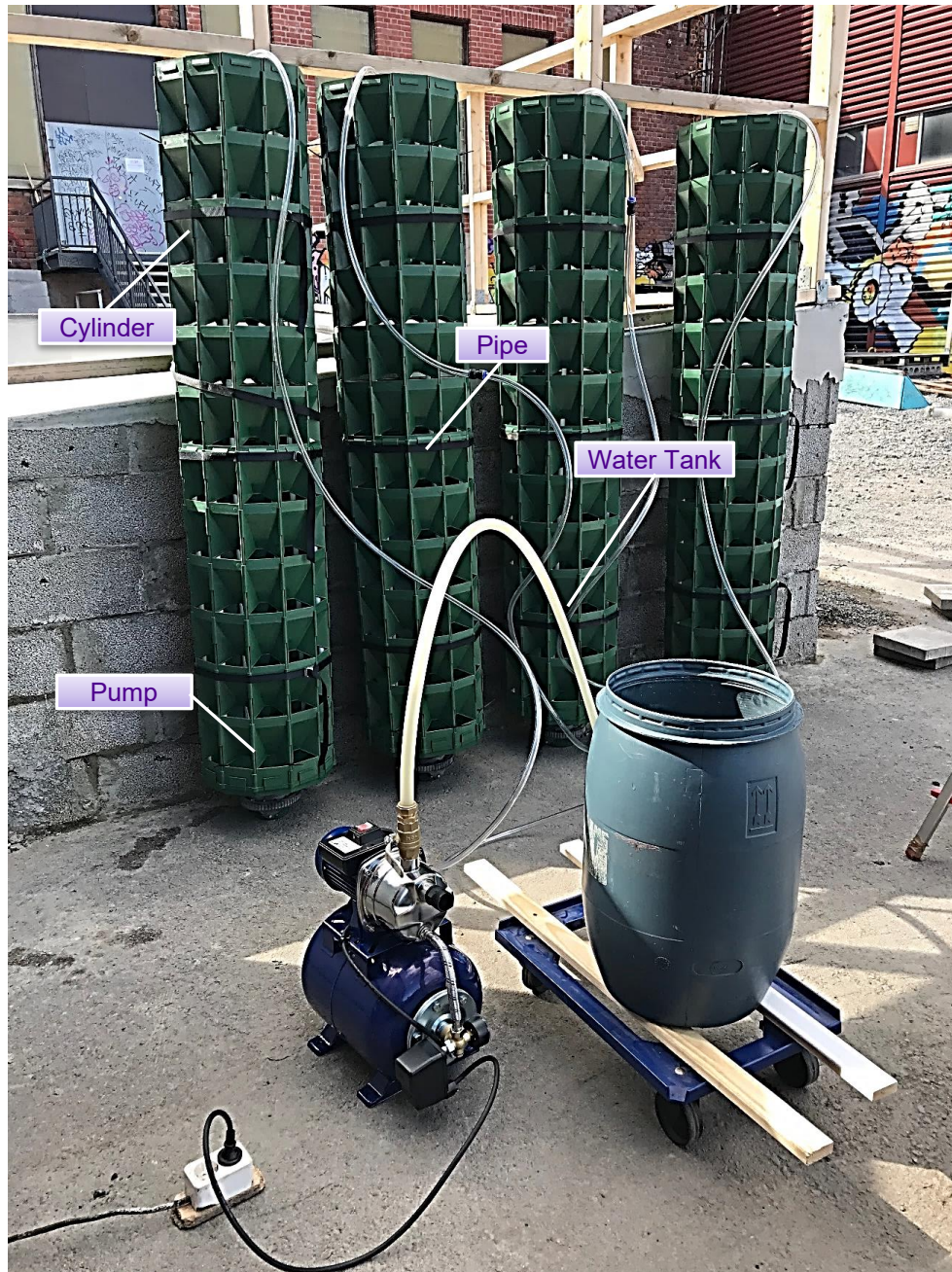
PICTURE 2. Pump pressure and nutrition flow testing (Author 2019)
