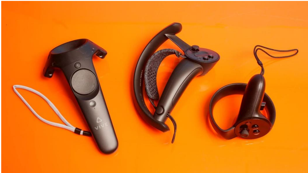
Picture 3. Different VR controllers from left to right: HTC VIVE, Valve Index, Oculus Touch. (cnet.com 2020)
