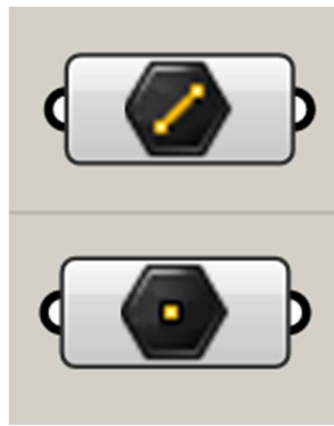
Figure 46. Nodes for importing lines and points from Tekla
