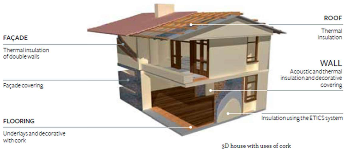
Figure 4. Illustration of parts of a building to which cork material can be applied (APCOR 2015f).
