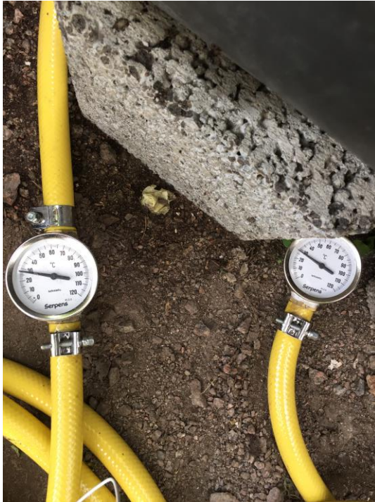
PICTURE 13. Inside glasshouse thermometers. On the right inlet water, on the left outlet water. (Author 2020)
