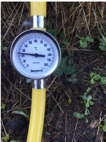
PICTURE 14. Thermometer for cold water coming to the compost pile reading 24°C (source: Author, 2020).
