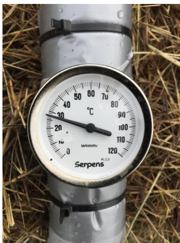
PICTURE 12. Thermometer on insulated hose at the outer edge of the pile reading 28°C. (Author 2020)
