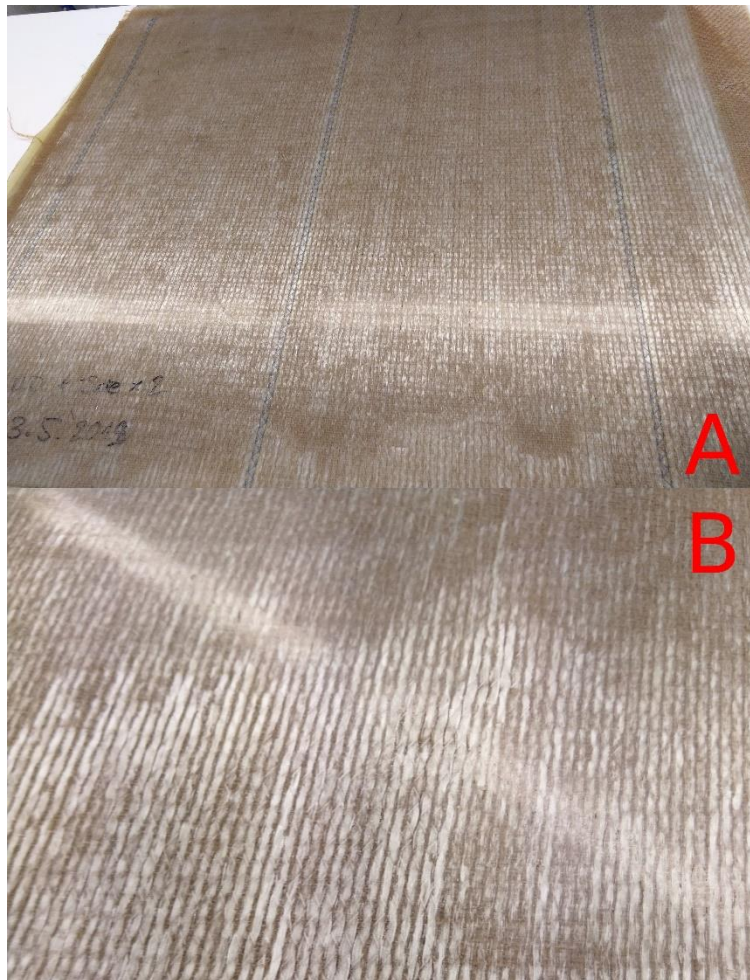
Figure 4.27 Sample 4 with UD fiberglass and Jute. (A. Overview; B. Wettability problem)
