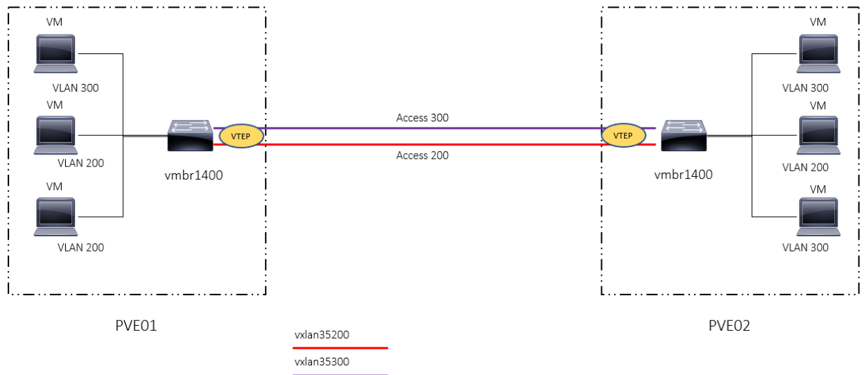
Figure 18 VLAN-aware bridge with VXLAN access
