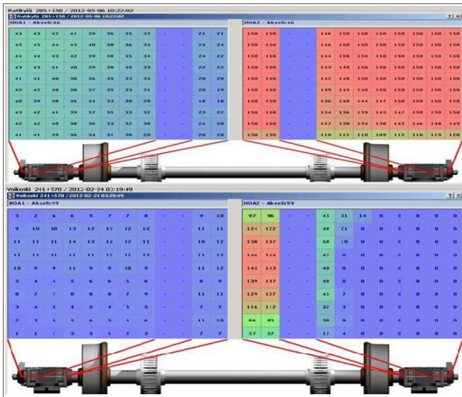
Figure 3. A temperature matrix is formed from the measurement results of the hot bearing detector (Liikennevirasto). (Junnikkala & Untinen & Haataja, 2016)
