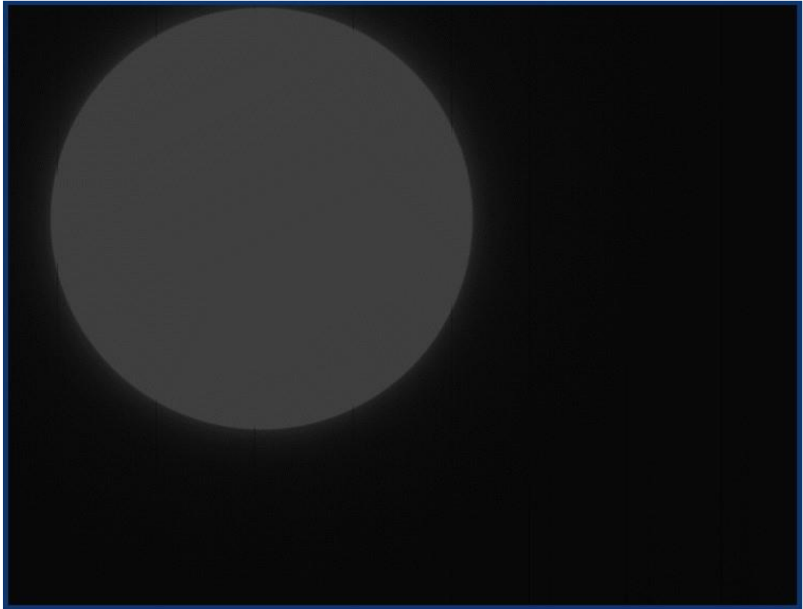
Figure 21. Test image with 0,02 second exposure time and a 2mm thick aluminum plate.
