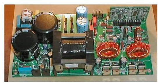
Picture 3.6 Power supply circuit (http://www.cadaudio.dk/paindex\_en.htm)
