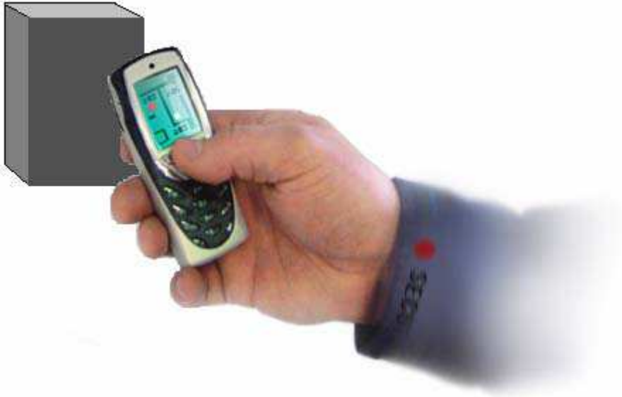
Figure 3. NFC server enables using a mobile phone as the user interface for non-UI devices. (VTT 2007, 34)
