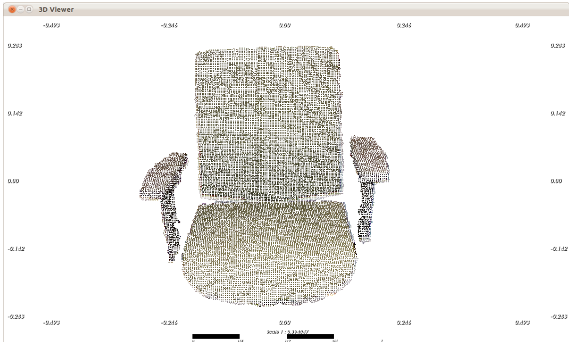
FIGURE 6. The final point cloud after all filtering methods are applied. The point cloud has 22539 points total in it.
