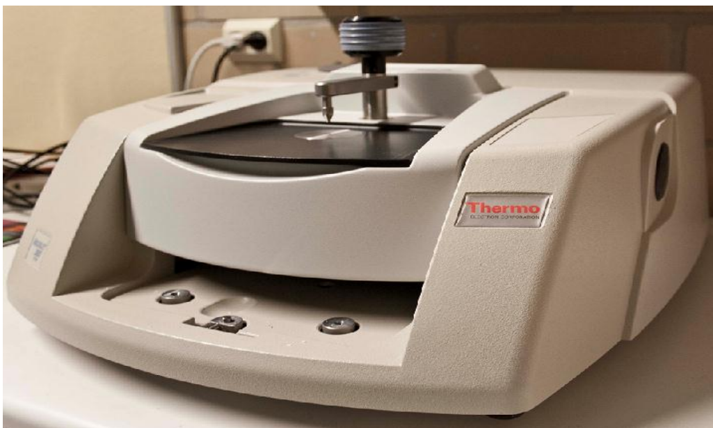
FTIR-laitteisto; Nicolet 380 FT-IR, Thermo Electron Corporation
