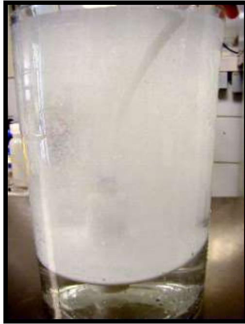
GRAPH 18. Fine bubble distribution of ceramic diffuser
