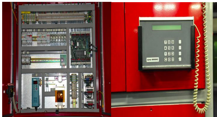
Figure 44 Alma Manu: Internal program in stacker
