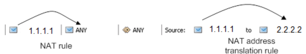
Figure 4. Network Address translation example. IP 1.1.1.1 connecting to any IP address and any service is translated to 2.2.2.2 IP address.
