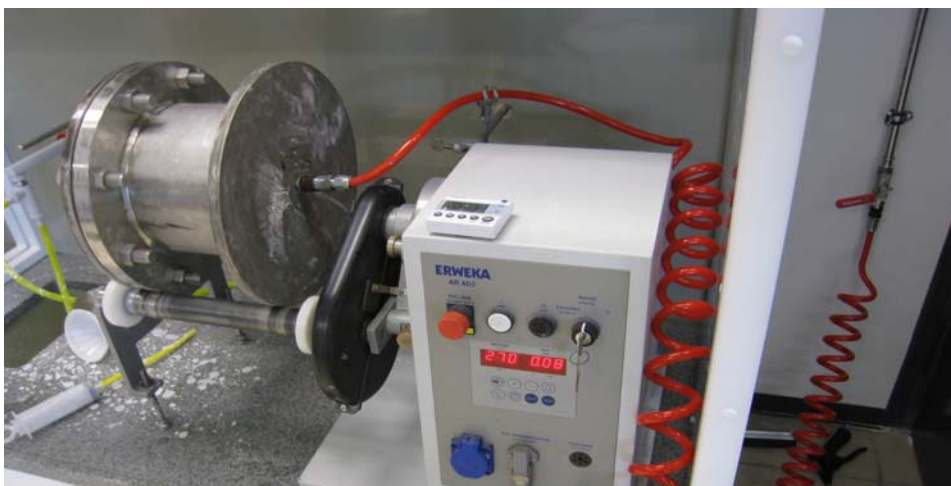
Figure 9 Rotating reactor with compressed air blast.
