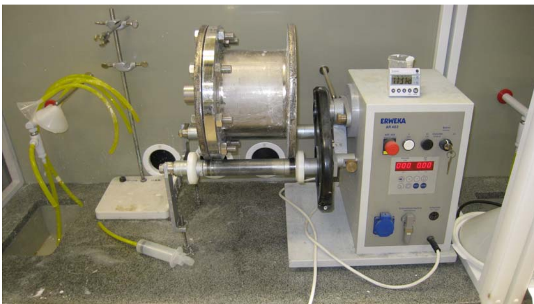
Figure 8 Testing arrangement with rotating reactor.
