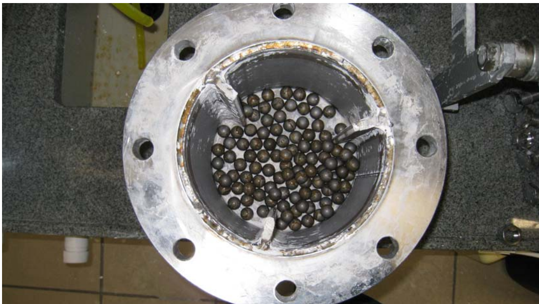
Figure 6 Reactor and grinding bodies.
