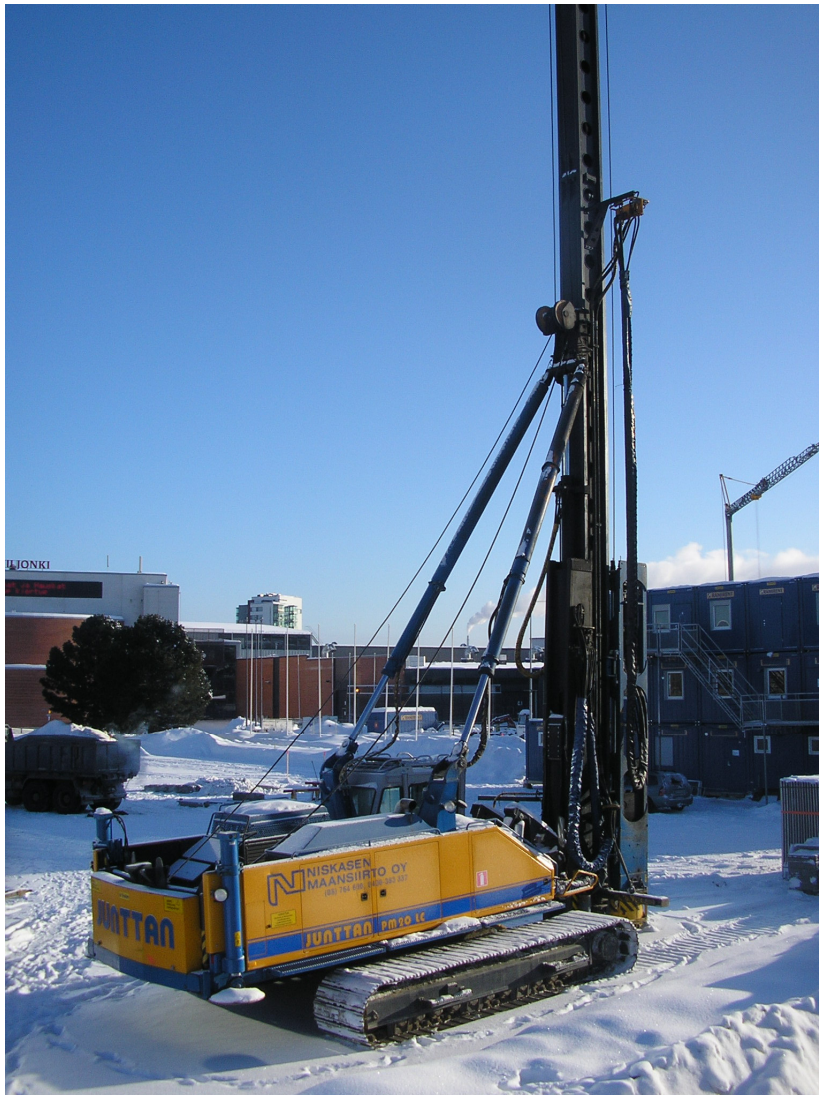
FIGURE 1. Junttan's hydraulic piling machine (Junttan Oy, 2012)
