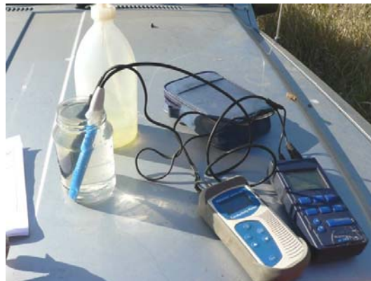
PICTURE 20. Conductivity and pH meter (Source: Liisa Pekonen, 2007)
