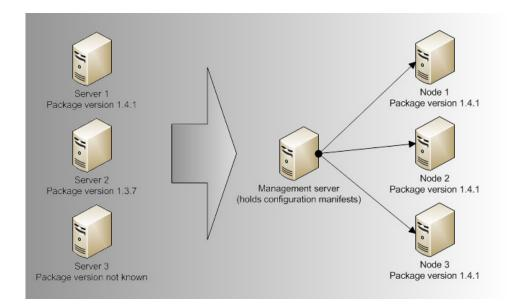
FIGURE 5. Using configuration management to manage packages
