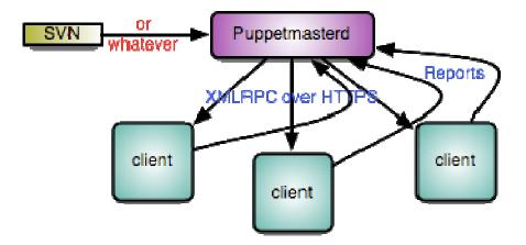
FIGURE 7. Data flow in a typical Puppet implementation (Source: PuppetLabs 2012)
