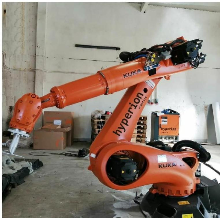
Figure 6. KUKA robot for 3D printing
