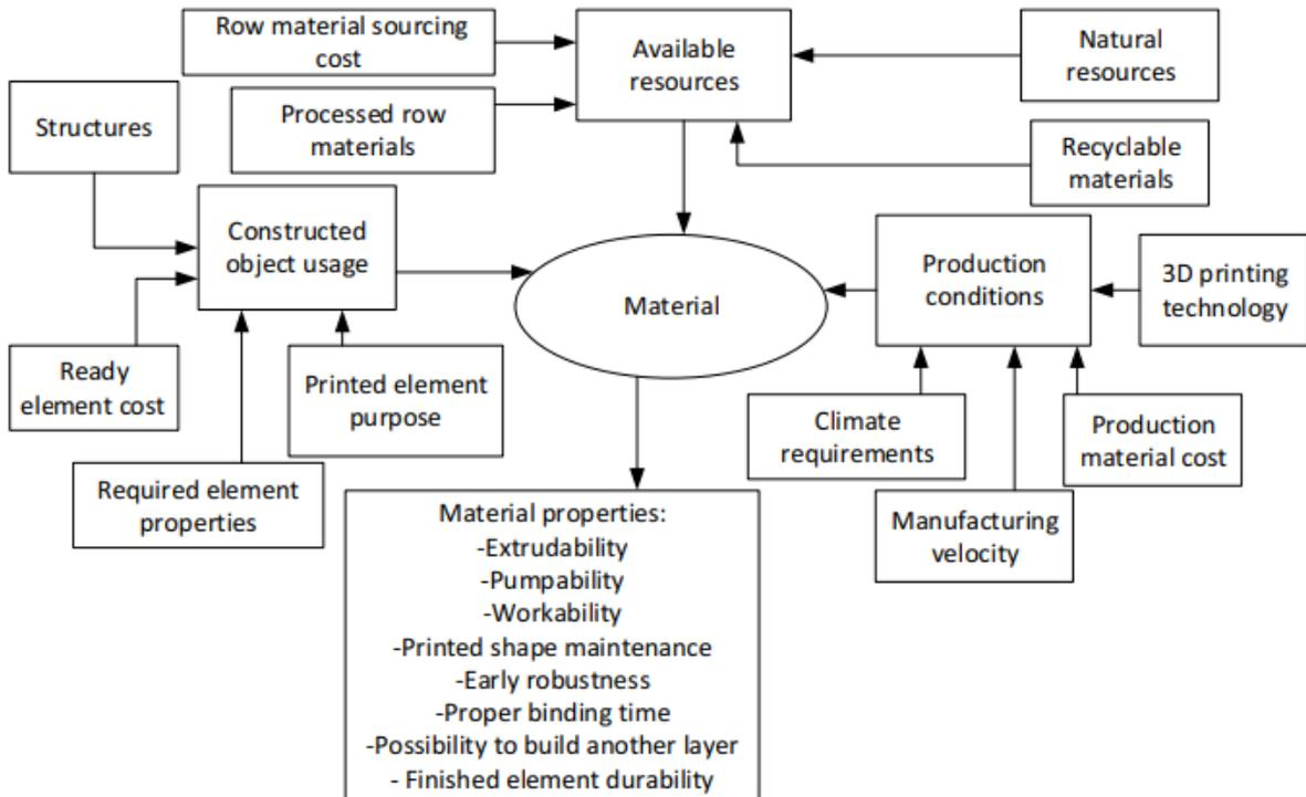
Figure 10. Building material composition for 3D printing and properties requirements
