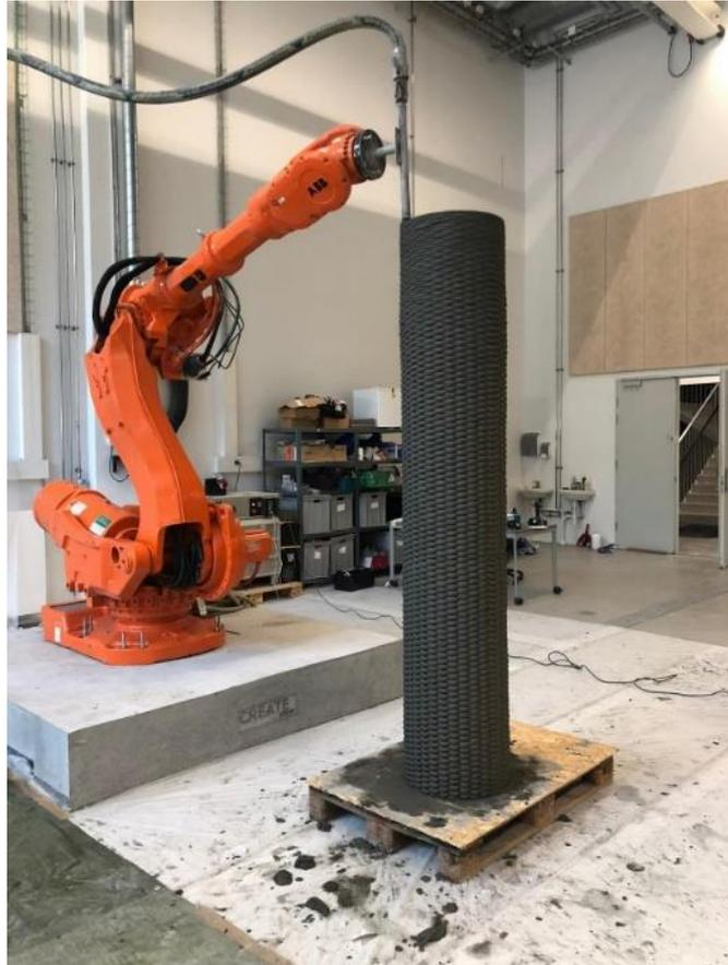
Figure 5. 3D printed concrete column made by Hyperion Robotics
