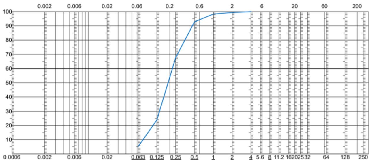
Figure 12. Sand particles distribution curve
