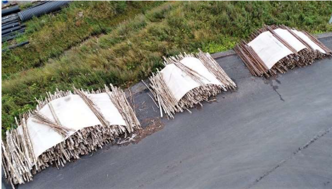
Fig. 5. A covered energy wood store at Kauhava heating plant. Covering was done for determining the production costs of dry wood chips.
