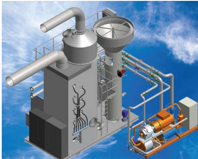
Fig. 2. Caligo flue gas scrubber and heat pump. The flue gas moisture of fresh wood acts as an effective heat exchanger when the flue gases are washed, and the energy is recovered in the heat transfer system ( www.caligoindustria.com )
