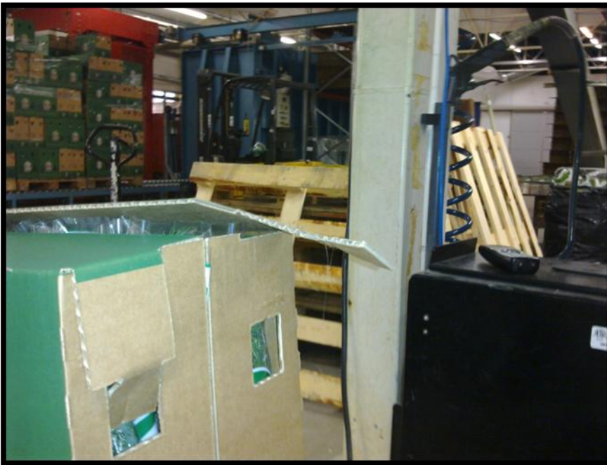
Figure 22. Glue failure after final packaging by WAM (Photo, Aduadjei 2011)
