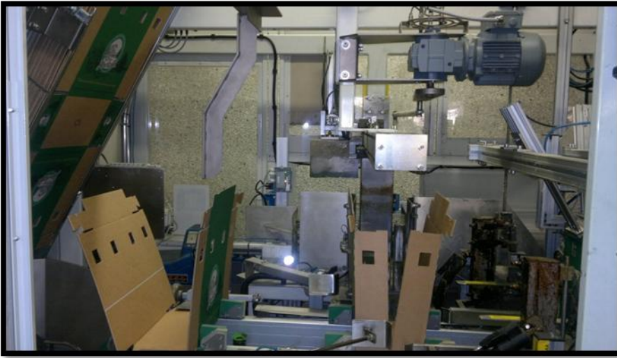
Figure 9 Skeletal Paper carton pulled onto the flight chains by the gripper (LHS photo) (Photo, Aduadjei 2011).
