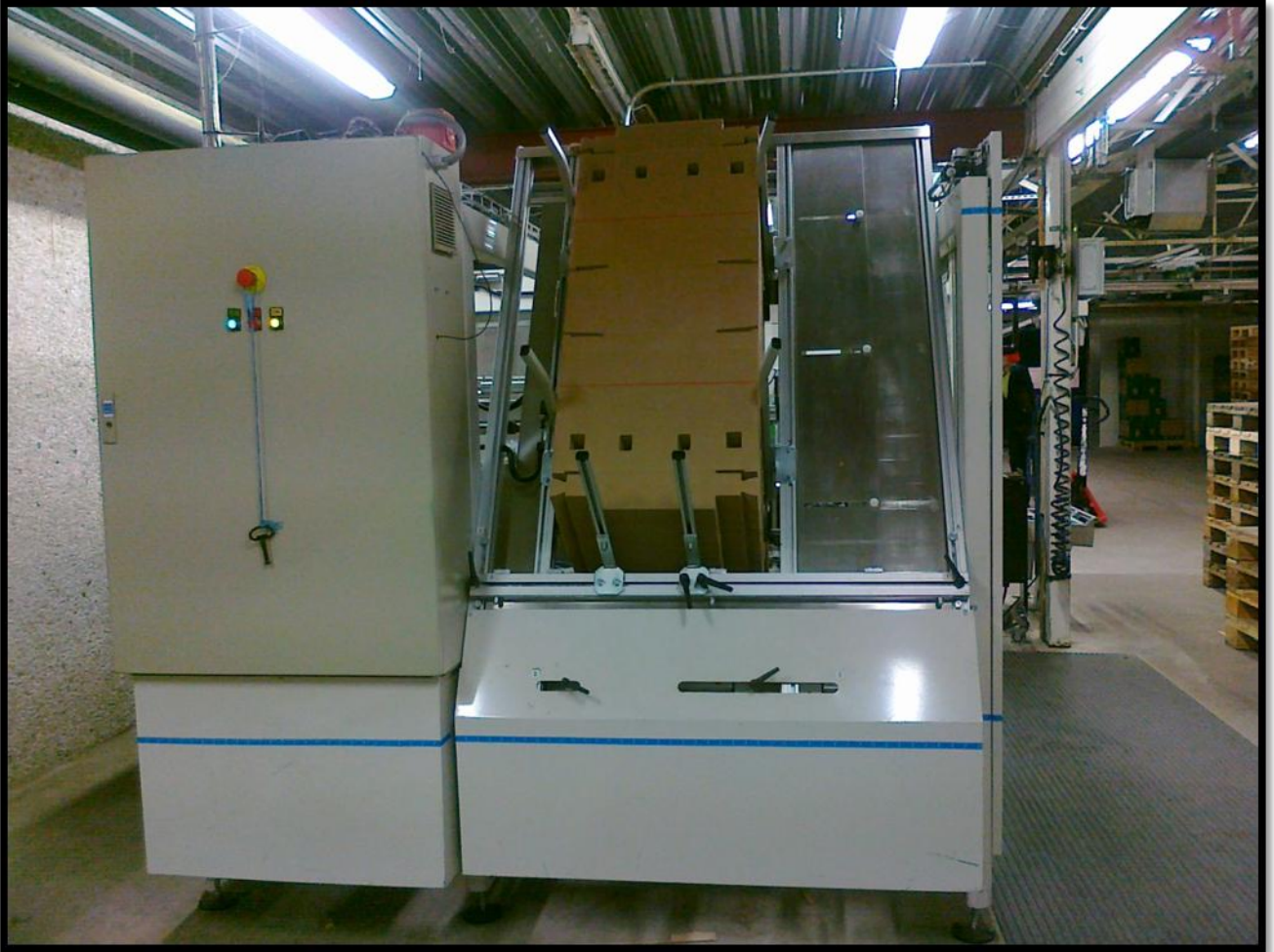
Appendix 2- Skeletal Paper cartons loaded at the back of the WAM (Photo, Aduadjei 2011)
