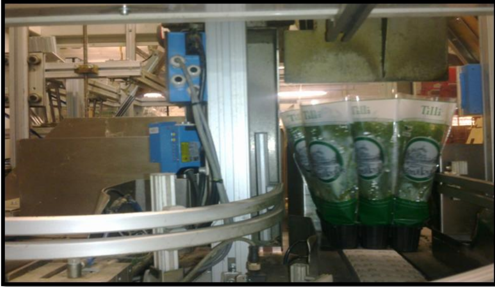
Figure 16. Barcode reader, reading a product group (Tilli) (Photo, Aduadjei 2011).
