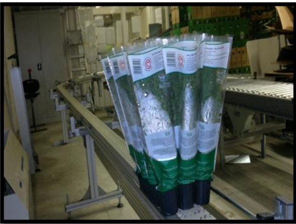
Figure 7 The recipient conveyor transporting a product group to the WAM (Photo, Aduadjei 2011)
