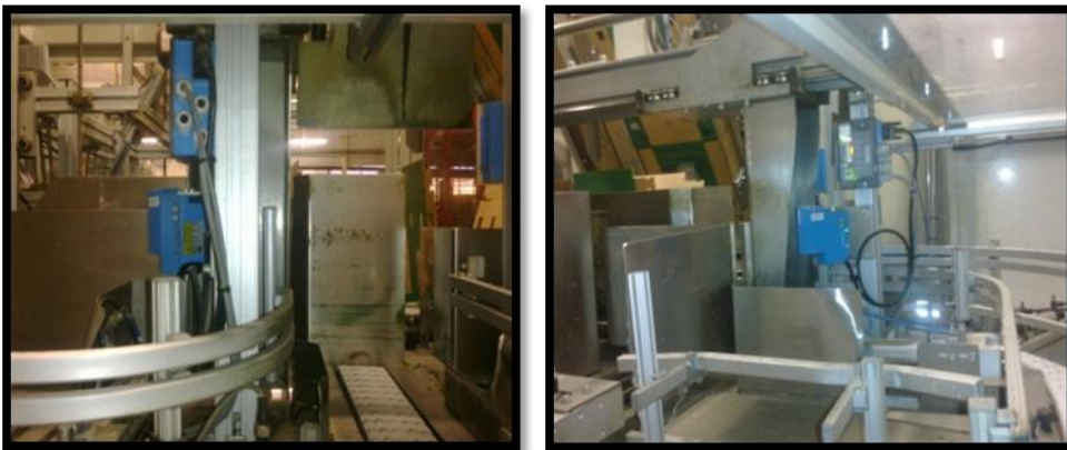
Figure 15 Barcode at Entrance of WAM (LHS) & Side View of Barcode Reader (RHS) (Photo, Aduadjei 2011).
