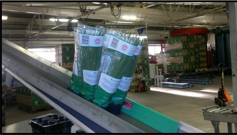
Figure 6 Production Conveyor transporting packed product group to the Recipient Conveyor (Photo, Aduadjei 2011)
