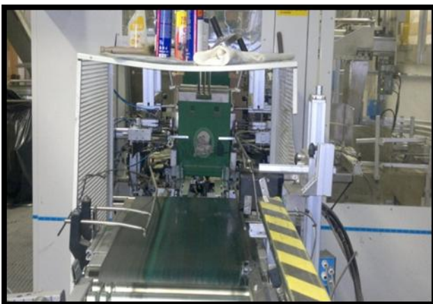
Figure 10 Packaged product at the Packaging Station waiting to be received by the Primary Delivery Conveyor (Photo, Aduadjei 2011)
