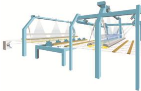
Figure 4.1.2.4 Strength grading and CE marking with using BoardMaster and EndSpy systems
