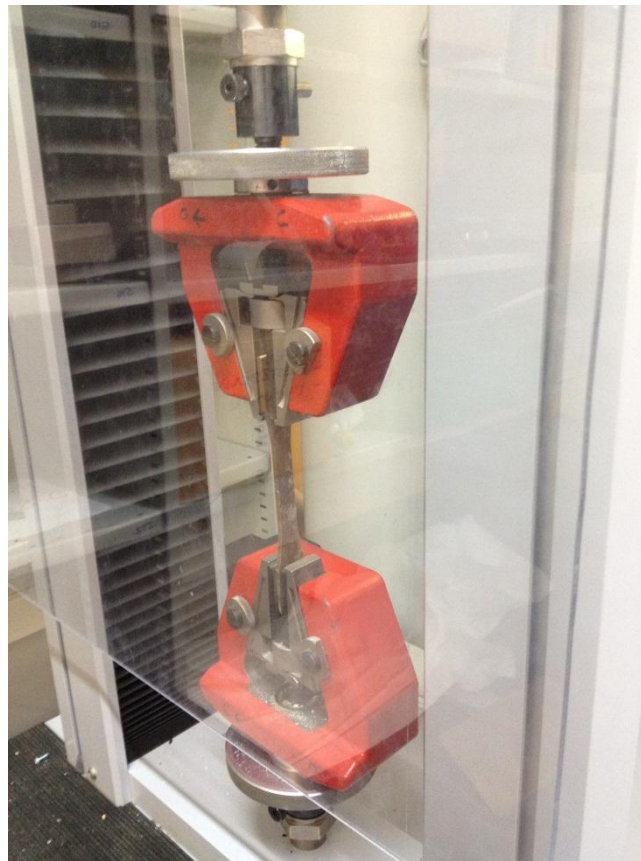
Figure 33 A dog-bone piece clamped to the Testometric machine for tensile testing
