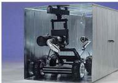
**Figure 34. Danduct robot in the duct. /13/**
