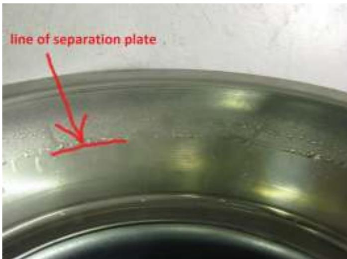
**Figure 30. Drops of liquid filtrated particles inside the turbo swing after the measurements.**
