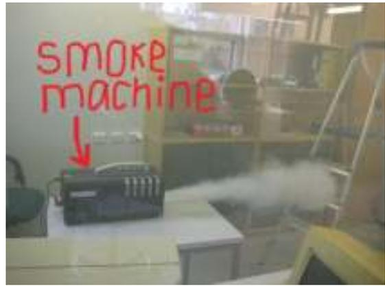
**Figure 17.** Smoke machine MAGNUM 1200 in MUAS laboratory.
