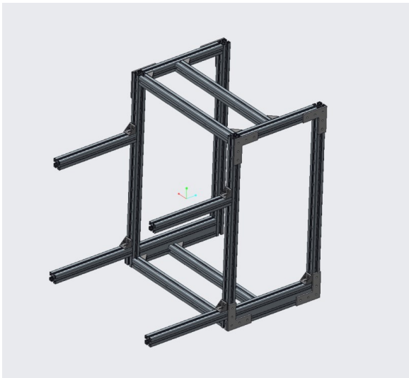
Figure 27. Frame of Painting System
