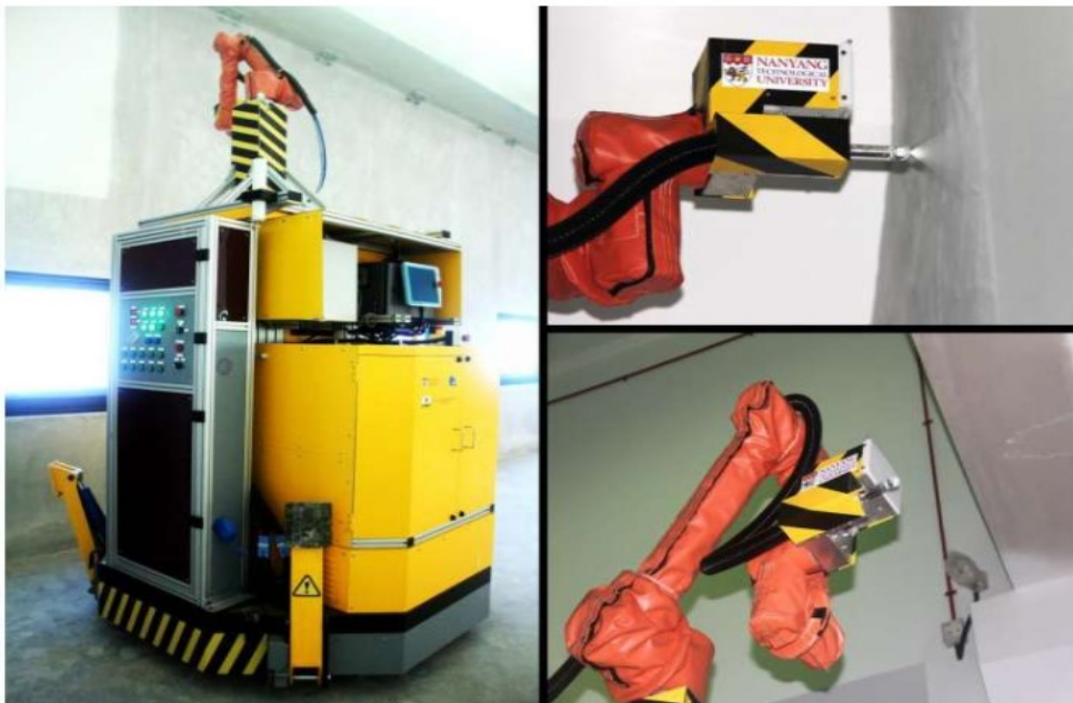
Figure 8. Wall Painting Robot (Nanyang Technological University, 2016)
