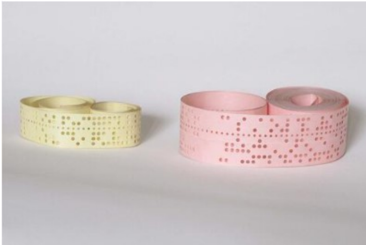
Figure 5 Programmed paper strips (Owen-Hill, 2016)
