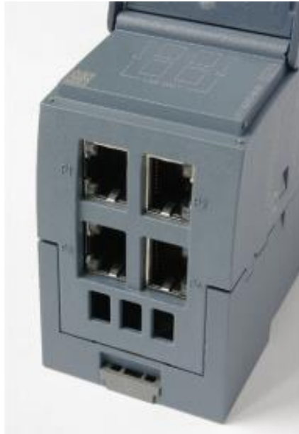
Figure 11. RJ-45 jacks of the CSM 1277
