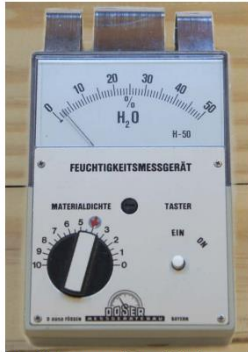
Fig. 12: Commercially available device using the capacitive method
