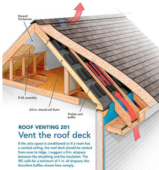
Figure 13. Roof deck ventilation (BuildingScience 2011)
