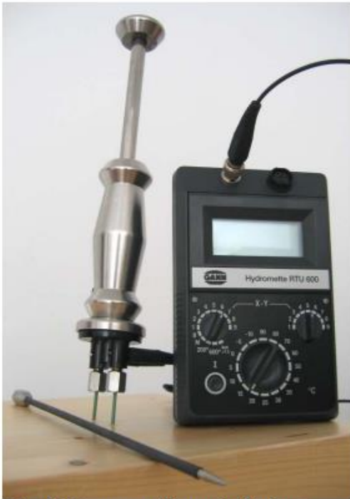
Fig. 11: Commercially available device using the resistance method
