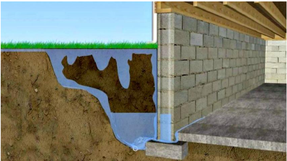
Figure 4. Basement Seepage after rain (Pinterest 2020)
