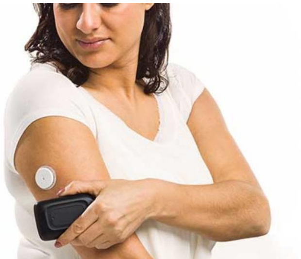
Picture 1. A blood glucose sensor and its reading device. (Diabetes-lehti 2016.)
