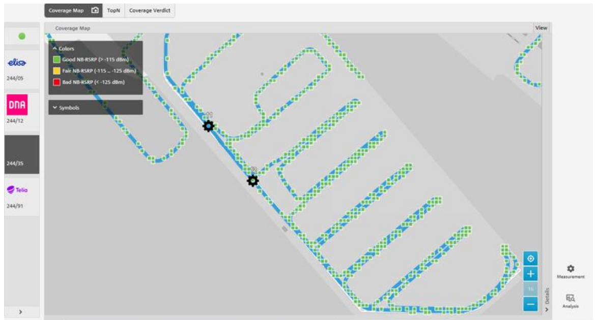
Figure 32. Coverage Analysis for pre-5G network within the container field (R&S@ROMES4)
