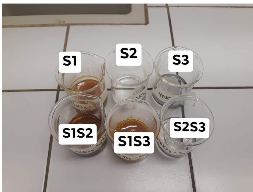
Picture 11: The corrosion of samples in \text{HNO}_3
