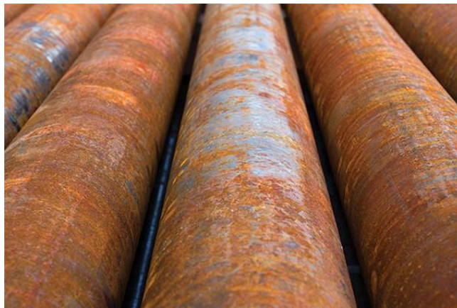
Picture 3: Uniform corrosion (Bardi, 2019)
