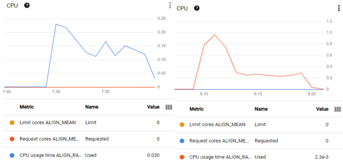
Figure 12. CPU usage of Go app (left) and Java app (right).
