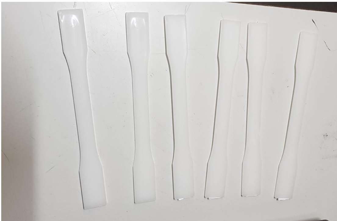
Figure 14. Polypropylene dog-bone sample
