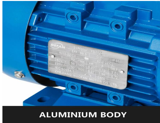
Figure 40. The three-phase motor nameplate of 0.37kW Defan Universal B3 Reprinted from eBay [online].
