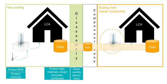
Figure 5. The data flow in the building process when reuse is included in the Peikko point of view.
