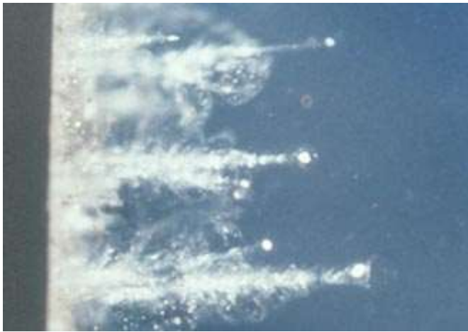
Figure 2 Comet dust trapped in aerogel 7
