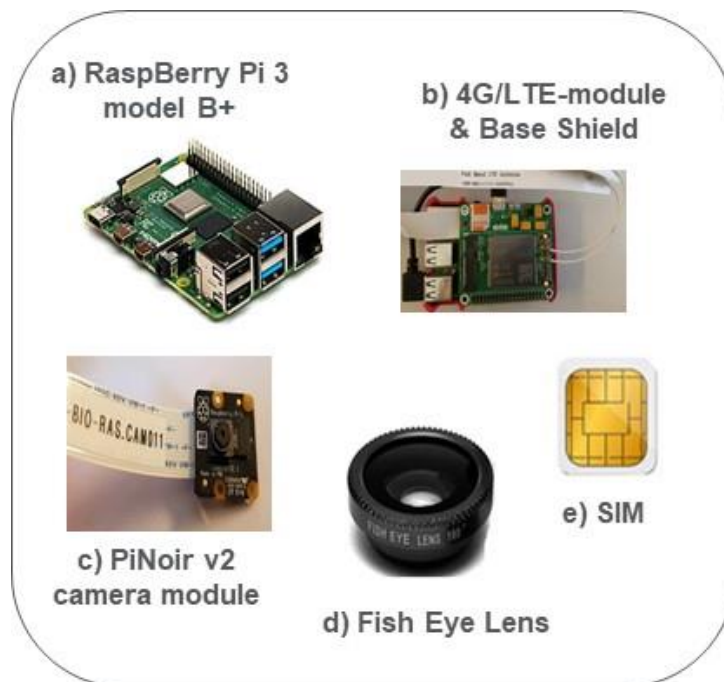
Figure 17: Components of the Raspberry Pi IoT-trap system
