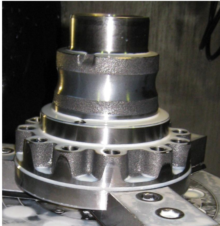
Figure 11 Bolt holes have been drilled in Dah Lih.
