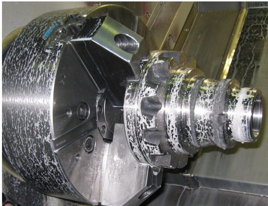
Figure 10 Machined part after the second Leadwell turning phase.
