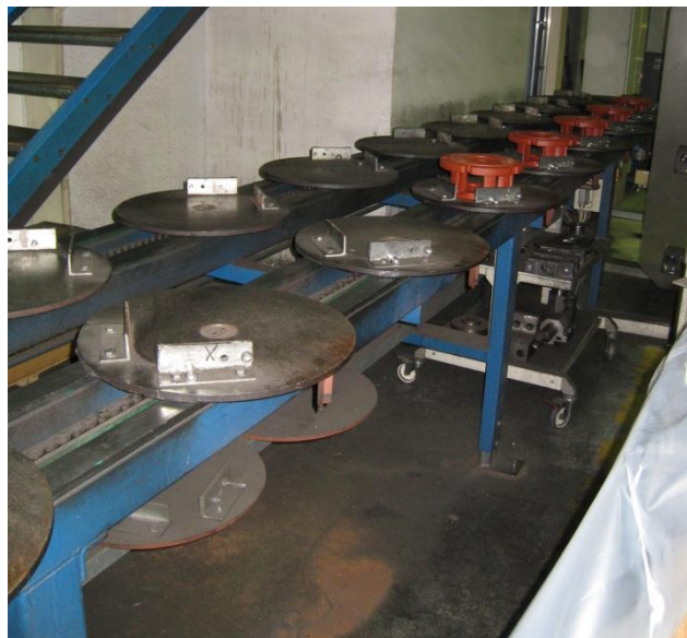
Figure 23 Conveyor system at robotized Sisu Axles Planetary carrier and – housing manufacturing cell.
