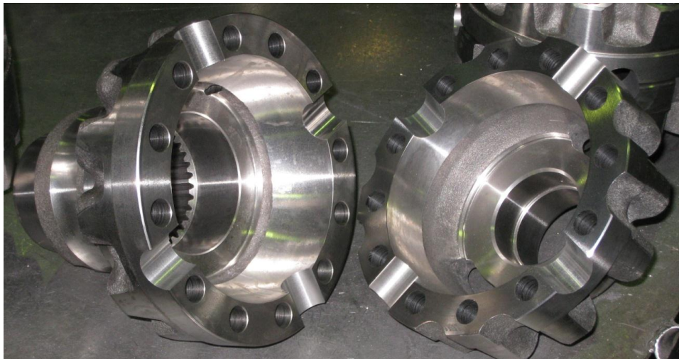
Figure 16 Cross shaft holes are drilled and the housing is ready for assembly.
