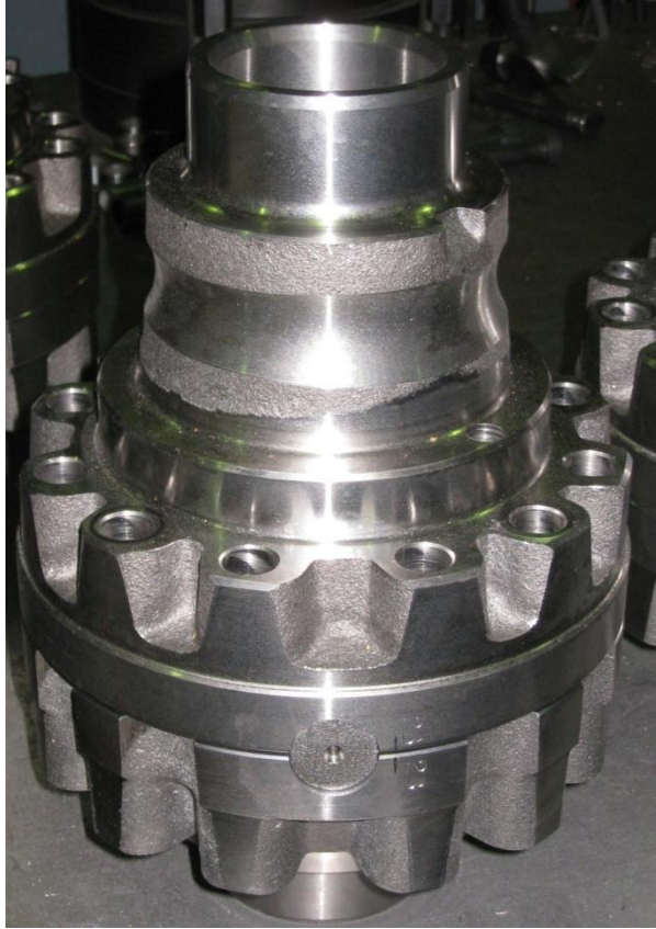
Figure 15 Cross shaft holes are drilled as an assembly. Note the lining stamp and numbering. The cross shaft fit is being tested.
