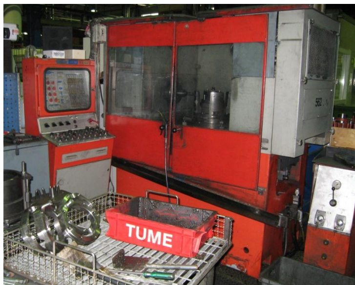
Figure 7 Lidköping PNF 23 cross shaft drill.
