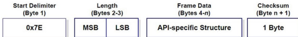
Figure 10. Structure of an API frame.
